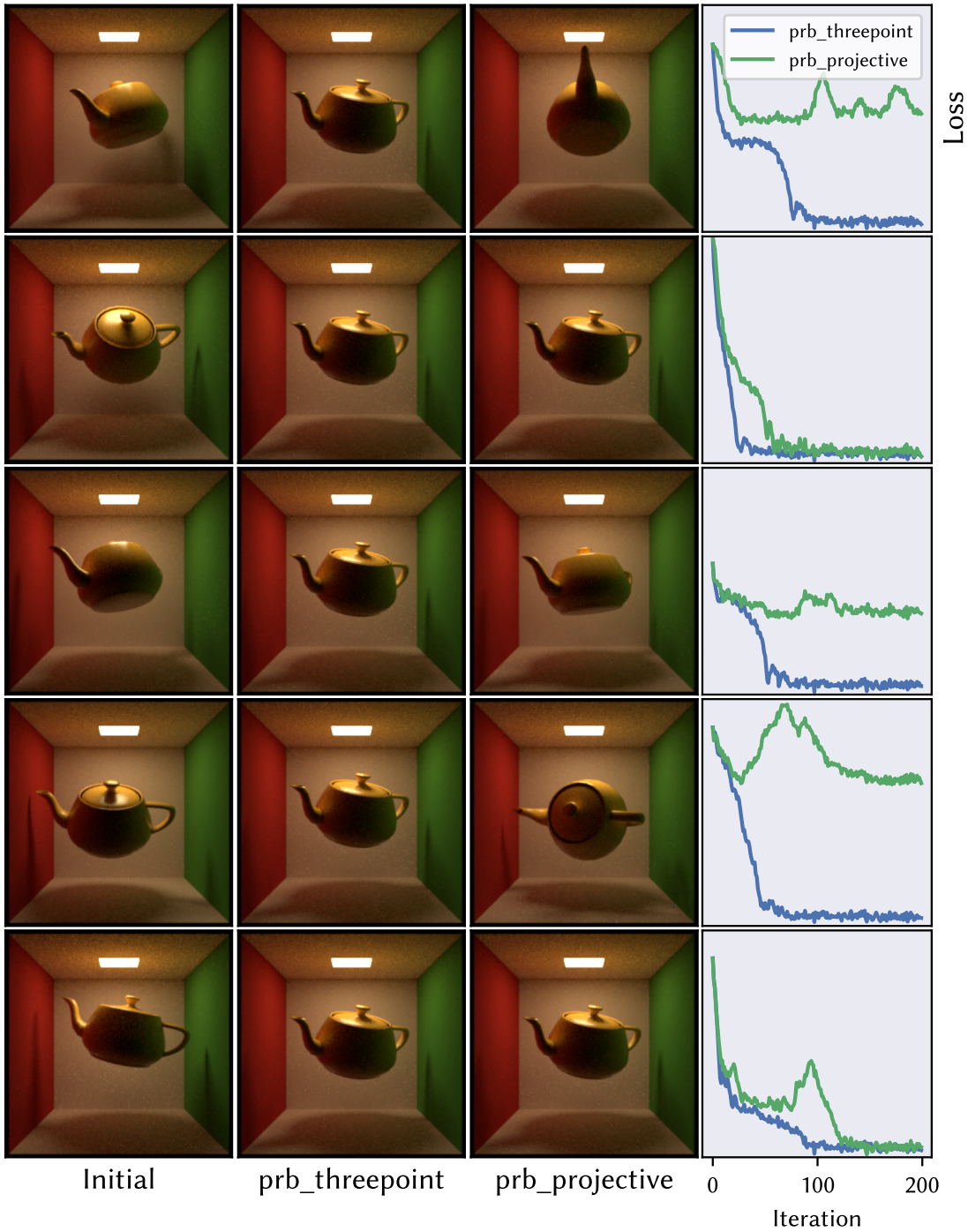
Figure 5.5: A simple inverse rendering task – recovering the 6D pose (position and orientation) of the teapot from a single image – fails if the interior derivatives are incorrect, even if discontinuities are handled ( prb_projective ). A radiative backpropagation-based implementation of the surface integral (Section 5.2.2) converges each time, despite not explicitly handling discontinuities ( prb_threepoint ).
